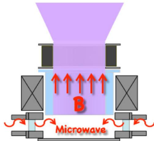
Fig. 1. (Color online) Solid-source ECR sputtering deposition system (JSW-AFTY AFTEX-6000). The substrate holder rotated during deposition and the temperature was varied using a ramp heater.
