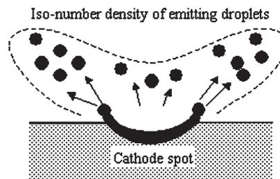
Fig. 1. Image of droplet emission from metal cathode spot.
