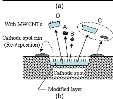
Fig. 2. Graphite cathode spot and image of droplet emission. (a) Graphite cathode spot (dc 50 A, no gas introduction). (b) Image of droplet emission of graphite cathode.
